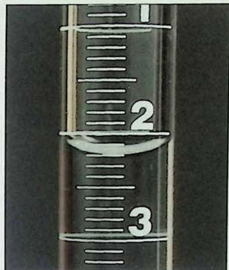
Figure 1.5. Reading the significant digits on a buret.
