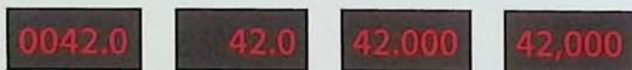
Figure 1.3. With digital instruments, all digits are significant except leading zeros. Thus, the numbers of significant digits in these readings are, from left to right, three, three, five, and five.
