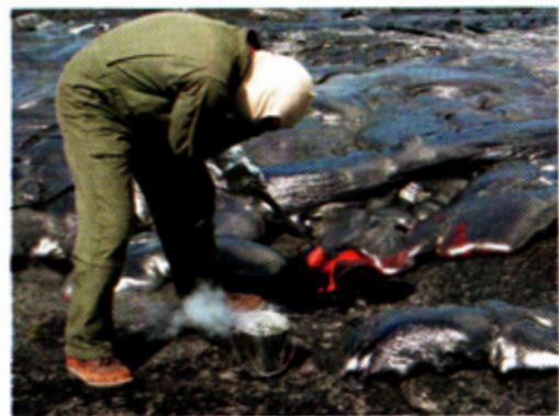
Figure 1.6. A geologist sampling 1150°C (2100°F) lava at Kilauea, a volcano in Hawaii.
